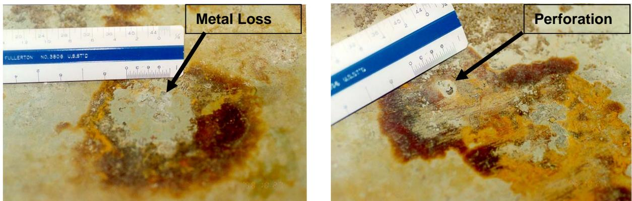
**Close-up Photos of MIC Corrosion on Stainless Steel Filtration Vessel Heads
