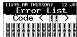
Pressing SELECT again while viewing any error code will clear all errors and generate an entry in the log.
