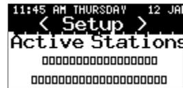
Pressing SELECT allows the user to scroll through individual menus which display if the station is enabled or disabled. The user can also exit to the previous menu.
