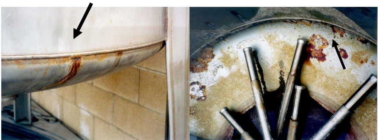
Failures of Stainless Steel Filtration Vessels by Crevice Corrosion (left) and Microbiological Corrosion (right)
