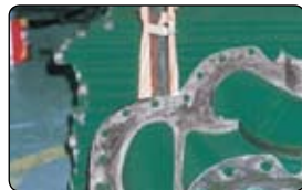
3 3M™ Scotchkote™ coating protects this pump housing from salt water and cavitation damage.
