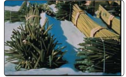
3M™ Scotchkote™ coated rebar ready for installation. 16
