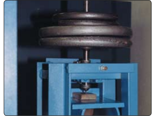
Gouge test simulates the stresses on a coating during a horizontal pipe pull. The coating sample is dragged under a weighted bit and the gouge depth is measured. Photo courtesy of Technical Inspection Services, Inc. (TISI), Houston, Texas 8
