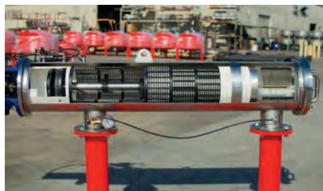
Twist-lock sectional screens provide easy cartridge replacement.
