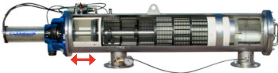
Filtaworx filters clean the screen filter based on pressure differential of inlet to outlet. During this cleaning event the screen is cleaned on both the out and return cycle.
